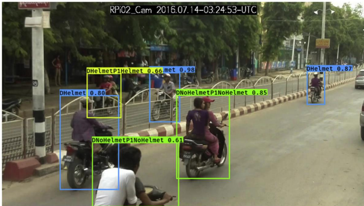
Computer vision based active motorcycle detection. This includes position specific helmet use registration (Siebert and Lin 2020).
